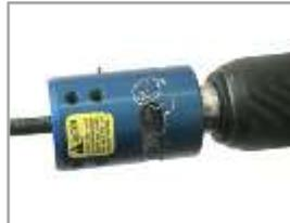
Actuate drill to remove jacket and expose center conductor. Then remove cable from tool.
