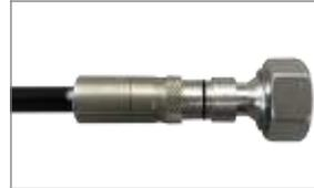
Thread connector onto cable until it reaches alignment mark and the connector bottoms on the cable.
