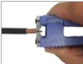
Use center conductor cleaner, SP-CC tool, to remove any remaining dielectric material on center conductor.
