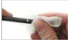
Use the alcohol wipe to clean the inner and outer conductors thoroughly.
