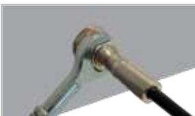
Mate the connector to the port, using the proper torque from the table to the right. When not attaching to a port, make sure the mating connector is supported by an adjustable wrench.
