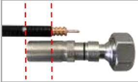
Align outer jacket end as shown with groove on the body. Mark cable jacket (using pen or marker) in line with end of connector.
