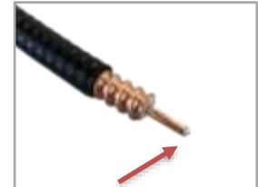
Proper prep is achieved when center conductor is chamfered as shown.
