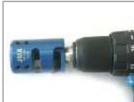
Attach prep/strip tool to drill. Be sure you are using an SP-14S tool.
