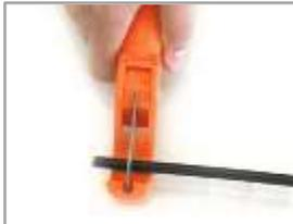
Straighten cable. Using RDCUTTER-S, apply even pressure while rotating tool around cable to cut off cable squarely.
