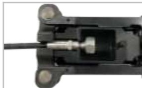
Make sure connector is fully seated. Press HCG trigger until compression tool cycles. Do not pull or push on tool during compression.
