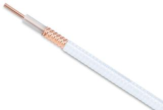
HL4-50, HELIAX® Plenum Rated Air Dielectric Coaxial Cable, corrugated copper, 1/2 in, off white PVC jacket
