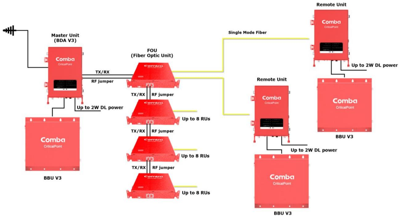
**NOTE: The V3 fiber DAS equipment is NOT compatible with the V1 Fiber DAS equipment**
