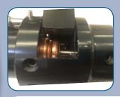
Gently pull back on cable to ensure tool is seated in a valley and the cutting blade is positioned over the valley closest to the end of the cable. Release blade lever and continue until cable is completely cut.
