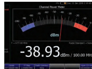
Built-in power meter
