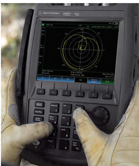
Large buttons make it easy to perform vector network analysis measurements—even with gloves on
