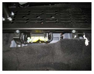
6. Attach Top Plate using 3/8-16 x .75 bolts and washers supplied in hardware bag.
