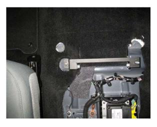
3. Attach Front Leg to center seat section mounting point, reusing original seat bolt or the M8 bolt supplied in the hardware bag.
