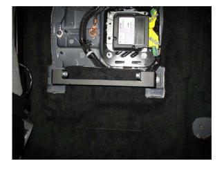
5. Attach Rear Leg to center seat section mounting points, reusing original seat bolts or the M8 bolts supplied in hardware bag.
