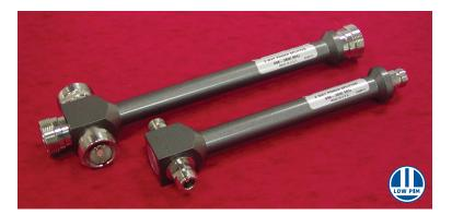
Microlab Model Dx-16 series of 2, 3 and 4 way Power Splitters has been designed to evenly split high power cellular and WiMAX signals with minimal reflections or loss. All joints are moisture sealed to meet the IP67. The mechanical shape allows easy attachment to wall using the supplied clips.
