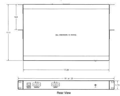
Fig. 1 Series 1720 Overall Dimensions (rear-panel connections shown with optional auxiliary contacts for indication of output status)
