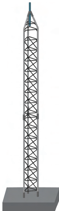
Typical Self-Supporting 25G, 45G and 55G Tower
