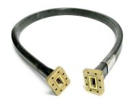
FlexTwist® Flexible Twist for WR137, 6.425–e 7.125 GHz, with interface types CPR137G and CPR137G, 900 mm
