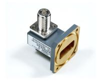
Waveguide/Coaxial Cable Transition for WR137, 5.85–8.2 GHz, with interface types N Female and CPR137G, gray
