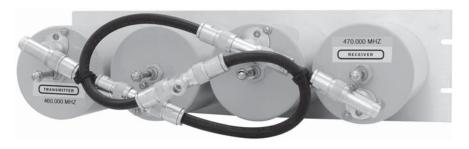
TPRD-4544/4744 duplexers mount on a 19" standard rack, with panel height of 5.25". Power handling is 250 watts. Receiver desense protection is at least 90 dB, and TX sideband suppression is at least 75 dB.
