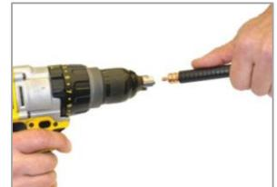
Use the coring bit "U" to remove dielectric until cable reaches stop on tool. You may optionally use the included T-handle to prep/strip & core cable.
