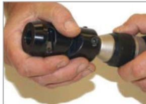
Attach the prep/strip tool to the drill. Be sure you are using an SP-1/2-LDF4D tool.
