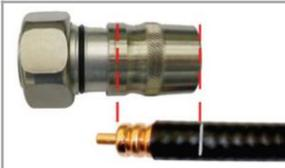
Align the outer conductor as shown with the groove on the cap. Mark the cable jacket (using pen or marker) in line with the end of the connector.
