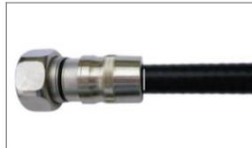
Push the connector onto the cable until it reaches the alignment mark, and two clicks are heard/felt.
