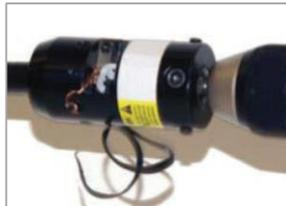
Actuate the drill to remove the jacket and expose the center conductor, then make sure the final cut is in the valley.
