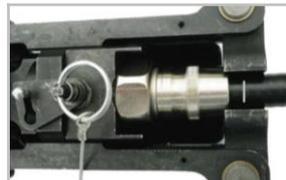
Make sure the connector is fully seated. Press the HCG tool trigger until the gun cycles. Do not pull or push on the tool during compression.
