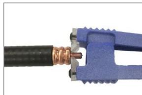
Use center conductor cleaner (SP-CC) tool to remove any remaining dielectric material on the center conductor.
