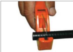
Straighten the cable. Using RDCUTTER-S, apply even pressure while rotating the tool around the cable to cut off the cable squarely.
