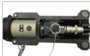
Select the proper insert for the connector. Pull/push back the insert to allow the connector/cable to lie flat in the frame.
