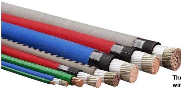
The economical KS-24194 non-halogenated copper wire is flame-retardant, low smokeemitting, and recommended for use in 600 V RHH\* telecommunication power plant applications.
