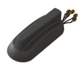
The Laird VFP69383B22JN multiport/multiband antenna provides an excellent solution for Public Safety, Transportation and Aftermarket Fleet applications. Configured for 2-port MIMO operation over the 3G/4G/ISM/CBRS bands and 2-port MIMO operation over the low//high frequency Wi-Fi bands. An additional 5<sup>th</sup> port provides an active antenna for enabling GNSS global navigation services.
