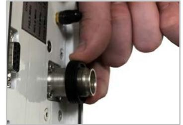
Install port seal, with text "This side away from nut" toward port.
