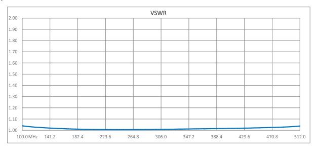
Click the following link (or enter part number in "SEARCH" on website) to obtain additional part information including price, inventory and certifications: 7/16 M/F Coaxial RF Surge Protector, 100MHz - 512MHz, DC Block, 750W, IP67, .5uJ, 20kA, Filter, Low PIM -155 dBc, Bracket Down, Hole Mount VHF50ED-MA-PGR
