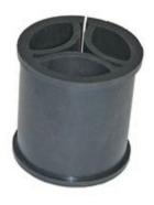
Grommet - Universal barrel cushion for 14-25 mm cables, for 1-1/4 in Standard or Click-on Hanger
