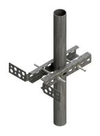
PIM-guard Antenna and RRU Cable Support Bracket with 8 ports for stackable hangers (up to 3 per port). Install with torque wrench set at 10 to 15 ft-lb to meet carrier PIM requirements. For patents, see www. cs-pat.com
