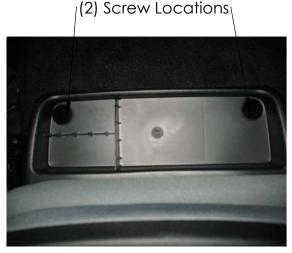
FIG 1 - Front Tray Removal
