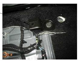
FIG 3 - Front Driver Bracket
