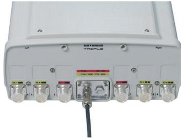
Connect a control cable to the daisy chain input of the FlexRET. The tightening torque for fixing the connector must be 0.5 – 1.0 Nm ('hand-tightened').
