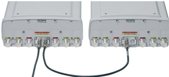
For daisy chain operation, remove the protection cap and attach a control cable to interconnect with the daisy chain input of the subsequent FlexRET or external RCU.
