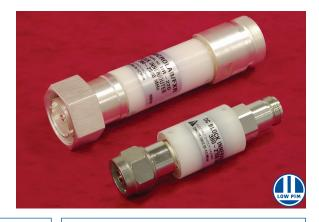
These DC Blocks are used to prevent the flow of direct current and low frequency current surges along the inner and outer conductors of a transmission line, while permitting the unimpeded flow of RF signals. Applications include the blocking of current surges in subway tunnels and at antenna sites during lightening storms. HR-21 series is similar except only the outer conductor is blocked.
