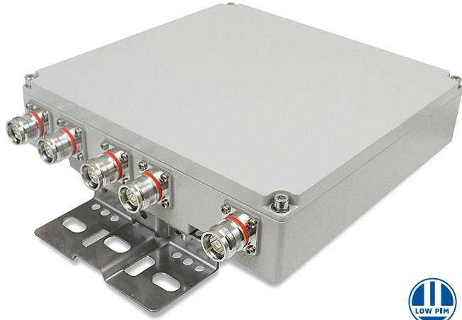
Microlab BK-5001E is a Pentaplexer which allows combination and separation of the signals in 617-798 MHz, 817-894 MHz, 1850-2000 MHz, 1695-1780/2110-2200 MHz and 2305-2360 MHz commercial wireless bands. To minimize band inter-reaction, the inputs are well isolated and have minimal insertion loss over their respective frequency bands. Attention to mechanical design ensures guaranteed low passive intermodulation.
