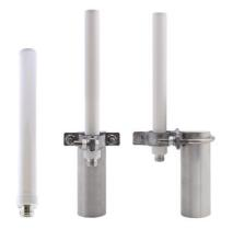
Laird Connectivity's OC35506P is a Low PIM omnidirectional, collinear antenna especially designed to complement interior or exterior mounted wireless networks operating over the CBRS band 3550-3700 MHz. An integrated RF connector is embedded in the antenna base cap for direct AP mounting. It comes complete with mast mounting hardware and includes a UV-stable radome enclosure that provides years of use without degradation to either mechanical properties or aesthetics.
