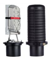
FOSC<sup>™</sup>450 BS Fiber Optic Splice Closure, Gel Cable sealing, no preinstalled tray, 6 cable attachments, with test valve
