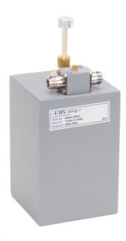
EMR Pass notch cavities are designed to allow a specific frequency or group of frequencies (pass band) to pass through the device while providing high rejection against a specific frequency or group of frequencies. These cavities may be factory tuned to specific frequency and are field tunable. Multiple cavities may be connected for greater selectivity with minimal insertion loss. Multi-cavity configurations come standard with 19 inch EIA rack mounting bars or panel with chassis tray.
