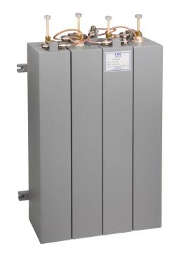
EMR pass-notch duplexers allow for the simultaneous use of a transmitter and receiver on a single common antenna. Our signature square cavities provide greater Q while requiring less space than conventional round cavities.
